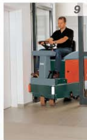
Hakomatic B910 with optional pre-sweep
